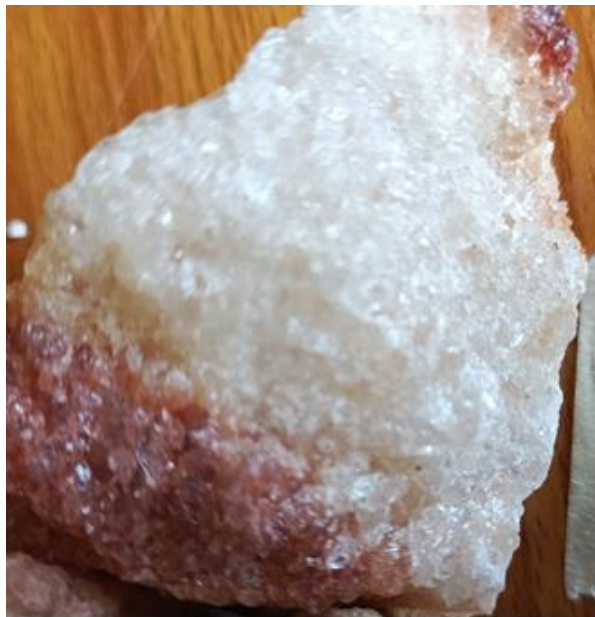
Figure 6: SP5: Quarze with Weathering (Hematization)
