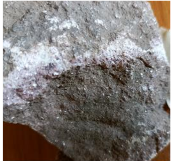
Figure 3: SP2: Lithium, Feldspar and Quartz
