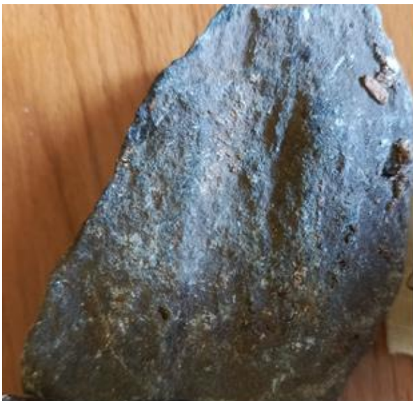
Figure 4: SP3: Gneiss with chloritization
