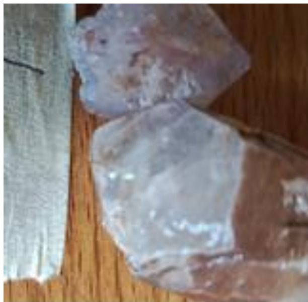
Figure 11: SP10: Quartz with stain of Feldspar
